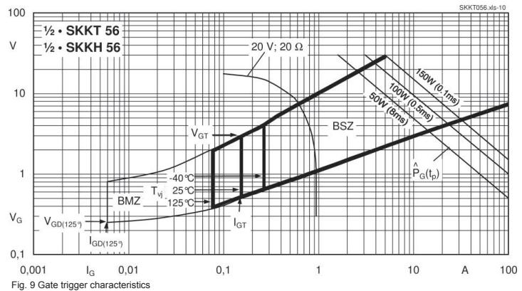
Fig. 9 Gate trigger characteristics
