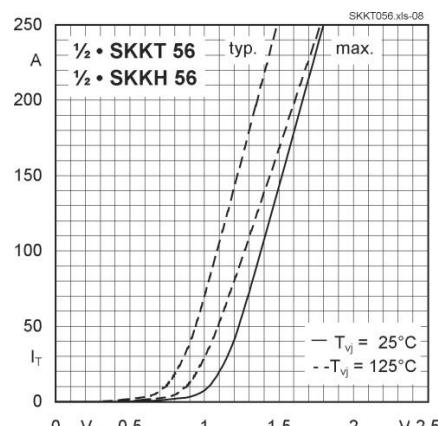
Fig. 7 On-state characteristics
